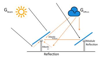
As outlined in the figure to the left, BFPV technology works by gathering irradiance from both the front and the back of a PV module. The technology provides increased generation from both direct and diffuse irradiation.
